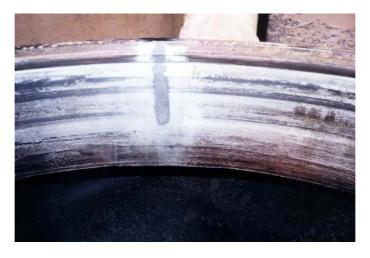
Repair of a marine engine with MM-metal SS-steelceramic and Hardener yellow. Damage: cracked packing surface between cooling water space and cylinder liner.
