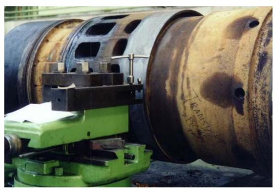
Repair of two-stroke engine cylinder liners Sulzer RND 76N ship's diesel engine with MM-metal SS-steel and Hardener yellow. The outer diameter is 900 mm and the inner diameter is 760 mm.
