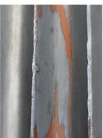
Several worn areas of a steel plant's leaky power transformer have been sealed with MM-metal oL-steelceramic and Hardener yellow.
