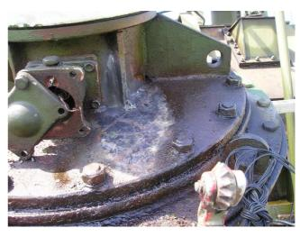
Repair of a vertical crack in a welding in length of  $\sim$  80 mm by using the repair technology "direct-MM-bonding" with the help of MM-metal oL-steelceramic and the hardeners red and yellow.
