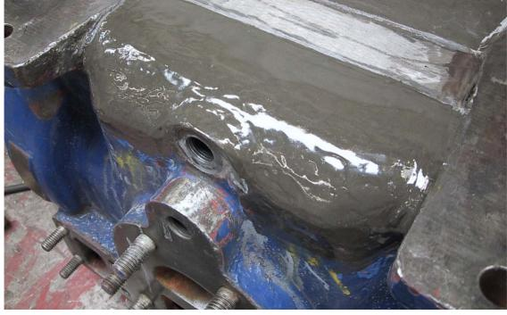
A broken pump casing was repaired with the help of the PolymerMetal MM-metal SS-steelceramic.
