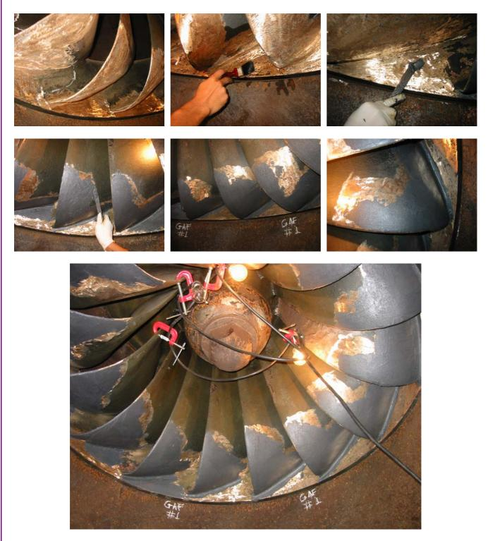
A turbine paddle was worn out caused by a water-sand-mixture. The pasty variant of the PolymerMetal Ceramium was used to rebuild the worn-out areas.
