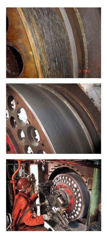
Onto a damaged area of an axle end MM-metal SS-steel, later MM-metal SS-steel 382 was applied to receive a higher surface quality. After curing, the work piece was machined down with a lathe to the desired diameter.
