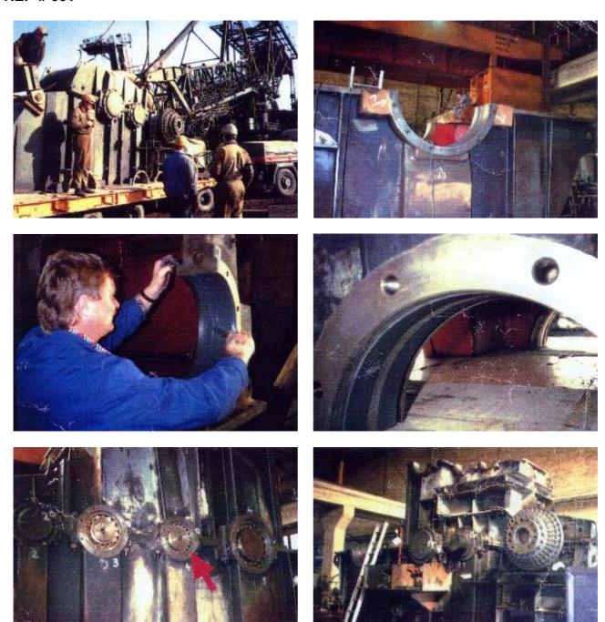
Repair of 14 bearing bushes of the gear box, which is destinated to the bucket wheel drive of an excavator for the field of open-cast mining. The worn bearing bushes with a diameter of 280 to 580 mm and a width of 130 to 150 mm were reconstructed with MM-metal SS-steelceramic and Hardener yellow. The standstill time of the excavator was considerable reduced to 72 hours.
