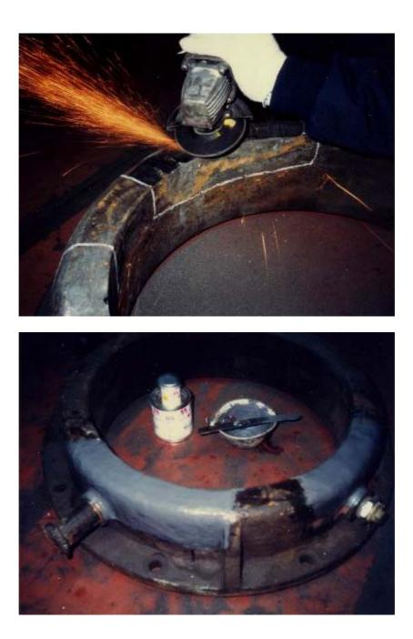
Corrosion damages at a brake drum caused by brake dust were repaired by using MM-metal SS-steelceramic and Hardener yellow.
