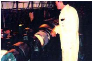
Repair of a paper roll with a diameter appr. 600 mm, length appr. 3400 mm and weight 8000 kg. Cause of damage: undersize of up to 1 mm at one journal bearing of 270 mm diameter. The repair has been carried out with MM-metal SS-steelceramic and Hardener yellow. After curing the roll has been machined with diamond tools.
