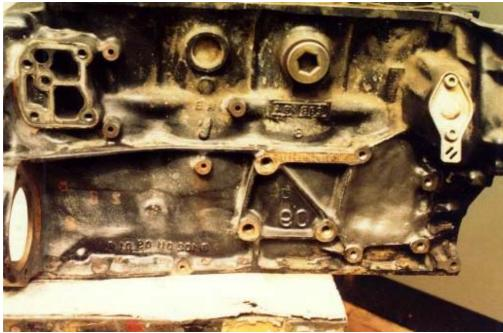
Repairing of a car engine Mercedes Benz near the crankshaft by using MM-metal SS-steelceramic and Hardener yellow. For reinforcement a 1 mm steel plate with the outline of the hole was patched into the engine.
