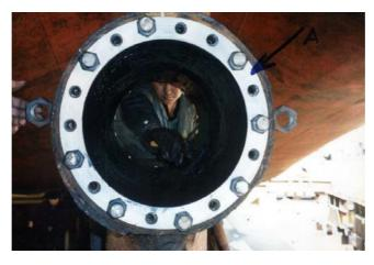
Repair of two tail bearings of a propeller shaft by using MM-metal SS-steelceramic, Hardener yellow and Hardener green. A ring with exact interior diameter has been bolted to both sides of the bearing. This ring has been centralized to the ideal shaft axis. Then MM-metal SS-steelceramic has been applied and been stretched parallel to the axis.
