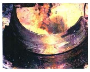
Repair of a grinding machine in a cement company. The damage, a worn out bearing housing, was repaired with MM-metal SS-steelceramic and Hardener yellow. Herewith the previous repair method "resurfacing by welding" was replaced.
