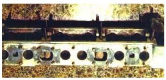
A cylinder head of a car engine having corroded under water channels was repaired by applying MM-metal SS-steelceramic and Yellow hardener.
