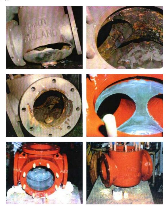
Repair of a three-way valve housing for sea water. Material: grey cast iron. Damage: considerable wash-outs as well as a gaping hole in the valve housing. The repair was carried out with MM-metal SS-steelceramic and Hardener yellow and Ceramium, liquid with Hardener CE.
