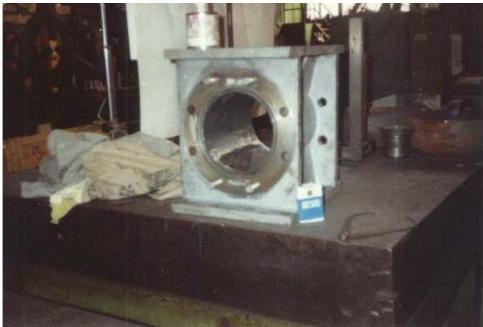
The upper part of an impeller of a pump for filling up the ready cement in sacks was exposed to very strong wear and tear. In the meantime it was tried to restore by build-up welding. The final repair has been carried out with Ceramium and Hardener CE.
