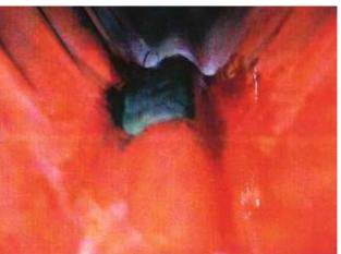
During the first run of a diesel locomotive's engine a shrinkage cavity in the casting was found above the engine block near the central lubrication. Oil was leaking from this cavity. The repair was carried out with MM-metal oL-steelceramic and Hardener yellow. After several test runs the repaired engine has been installed into a new diesel locomotive.
