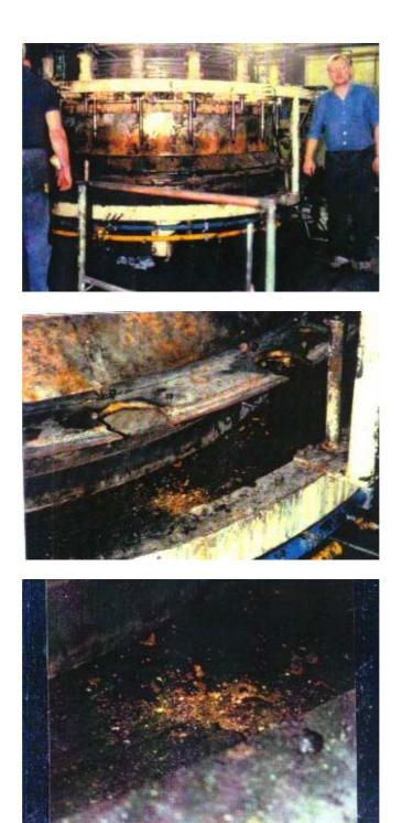
Repair of an automatic glass machine at a channel for broken glass and water. The coating procedure was affected in two steps - first application with Ceramium, pasty, followed by a second application with Ceramium, liquid. The previous reconstruction procedure was build-up welding.
