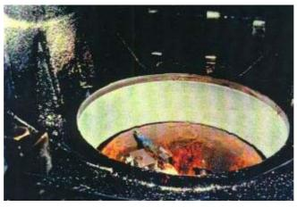
Through leakages at the sealing surface of a cylinder liner's engine block cooling water flew out. The reconstruction work was affected with MM-metal SS-steel and Hardener yellow at eight cylinder block threads. After the application procedure the seats were machined to nominal diameter 308 mm. The main engine was an engine Daihatsu type 8 DSM 26, power 1252 kW, 720 U/min.
