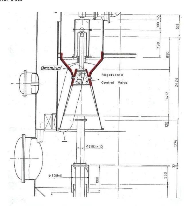
Ceramium with hardener CE was used to repair cracks and damages caused by erosion between cast segments at a gas washer (Venturi) of a blast furnace cleaning facility. Due to this the life of the component was doubled.
