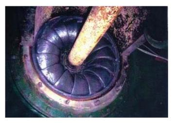
Repair of two turbine rotors. Damages were present at all areas of the blades where the water leaves the blades. First large holes have been welded. Then the erosive areas have been filled up with Ceramium, pasty. Finally a supplementary layer of VP 10-017 has been applied as protection against cavitation.
