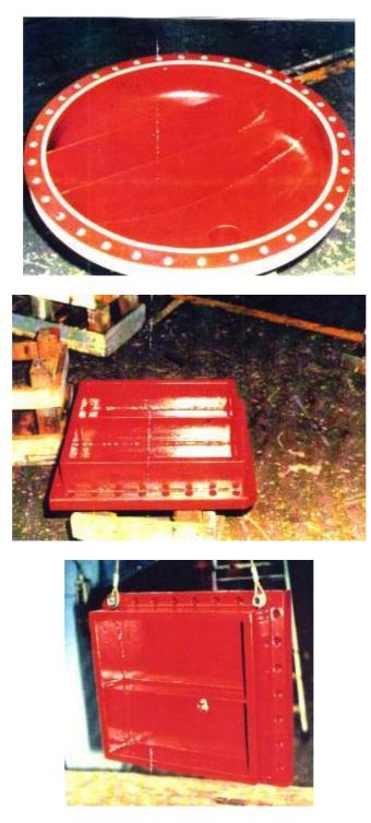
Various purposes of VP 10-017, a tough and elastic polymer-ceramic, which can be applied e.g. on covers, models, pump housings, mountings, pipe works, machines and plants. VP 10-017 offers a durable, elastical, high impact and wear resistant corrosive protection. VP 10-017 can be applied with brush or spatulas in one go to an application thickness of 300  $\mu$ m even on vertical surfaces.
