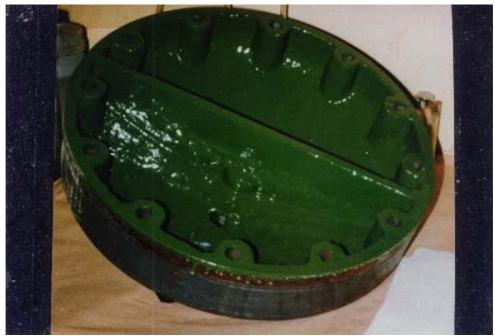
A cover with Ceramium was reconstructed. The coating was affected in two working procedures: First a surface reconstruction with Ceramium, pasty and Hardener CE. Second an application with Ceramium, liquid with Hardener CE.
