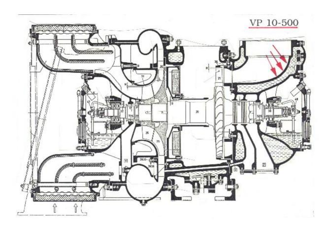
Repair of a ship's turbocharger with VP 10-500. Scourings, cracks and apertures from the gas entrance to the cooling water side were repaired with VP 10-500. For the reinforcement two layers of MM-Fabric tape (glass fibre) were used.
