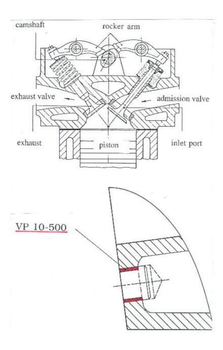
With VP 10-500 a non-sealant vent plug in a cylinder head at an exhaust port was repaired. VP 10-500 was applied in a thickness of appr. 3 mm. Afterwards the plug seals remained gas-proof in spite of high operating temperatures of 300 °C.
