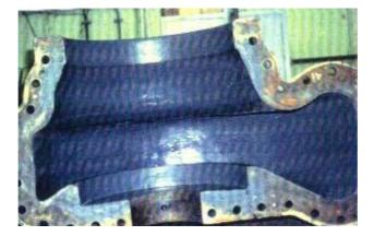
An additional water-centrifugal pump being damaged by erosion and cavitation was rebuilt using Ceramium. Housing and flanged socket were coated inside with VP 10-017.
