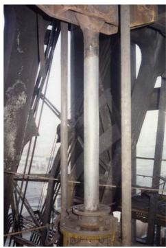
Repair of worn piston rods caused by the exhausts of a blast furnace. The piston rods were brought to nominal diameter again using Ceramium. After the repair has been completed the piston rods are in operation again over 3 years.
