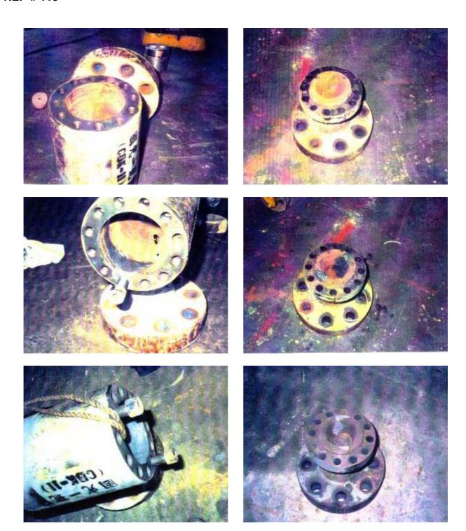
Repair of gas drilling surge valves. Abrasion due to escaping gas (2800 psi) and carrying contaminations such as e.g. sand. The repair has been carried out using Ceramium. A later inspection did not reveal any damages.
