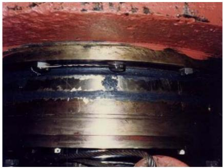
Repair of a leaking simplex compact packing. The repair was difficult due to oil pouring out of the repair site. Therefore it was decided to use the direct-MM-bonding method by applying the PolymerMetal directly on the greasy surface. Here MM-metal oL-steelceramic with Hardener red was chosen.
