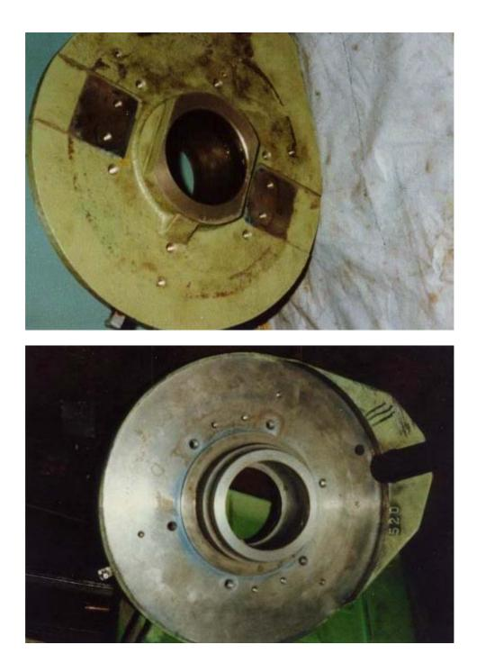
The bearing seat of a brake shield was reconstructed to its original size with Molymetall. First 2 mm were turned down and then Molymetall was applied. After total curing (appr. 12 h) the size of the original diameter of the seat was reached by turning down again.
