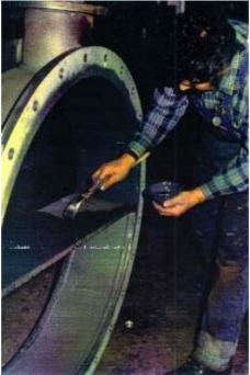
Durable protection against wear and corrosion on welded constructions e.g. receivers and covers can be achieved by using Ceramium together with an application of VP 10-017 afterwards.
