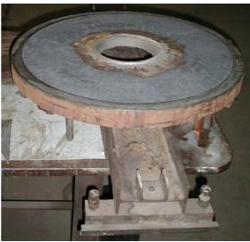
In a granulation plant several pumps (2 granulation pumps, 2 condense pumps, 2 cooling circuit pumps, 1 submerged pump) material loss caused by wear. All pump casings and running wheels consist of hard cast. Pumping medium is circuit water with a slag sand content of appr. 10 mg/l at a average corn size of 0,3 mm. The water temperature is 90 °C (194 °F) at the cooling circuit pumps and 40 °C (104 °F) at the condense pumps. The pumps have been repaired with a coating of Ceramium.
