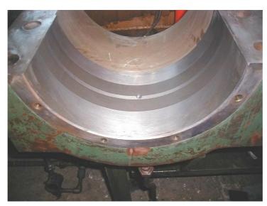
In a steel plant the repair of a broken gearbox with a weight of 40 t would have taken up 10 days by using the conventional way of welding. By using the repair technology of MultiMetall combined with the PolymerMetal MM-metal SS-steel and MM-Release agent a repair time of just 27 hours was necessary. Stresses of 120 MPa occur at the gearbox.
