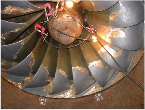
A turbine paddle was worn out caused by a water-sand-mixture. The pasty variant of the PolymerMetal Ceramium was used to rebuild the worn-out areas.
