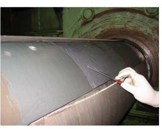
A reeling machine was worn out due to abrasion. After roughening the surface to be treated, it was coated with the PolymerMetal MM-metal SS-steel and therefore put into working order again.
