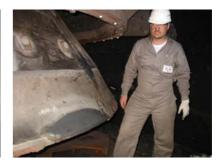
At a steelwork, heavy erosion caused damage of a blast furnace. Several areas of the conveyer cone were severely damaged due to the continuous loading with coke. Some plates were welded on the cone and then coated with Ceramium as well as some other damaged parts and the machine was put into operation successfully again.
