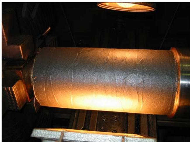
In a mining plant the cost and time intensive new acquisition of a replacement shaft for a damaged shaft of a vibrating screen was prevented by the repair with MM-metal SS-steel.
