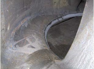
Due to abrasion a worn out metal ring of a dredging pump had to be replaced. With the help of MM-metal SS-steel the new metal ring was fixed. PolymerMetals present a high shearing strength; MM-metal SS-steel offers a value 30 MPa.
