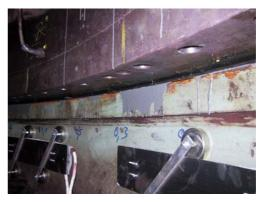
The slewing bearing ( $\emptyset$  4371 mm) of a bucket-wheel excavator showed some deviations outside of the tolerance range at some spots in the area between upper structure and chassis. For the solution of this repair problem the high-strength repair material MM-metal SS-steel 382 was chosen. The very thin fluid product type is extreme flowable and pourable.
